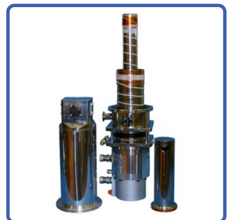
The above picture shows the DE210 Cryocooler installed on the GMX-20 interface with the vacuum shroud and radiation shield removed.
