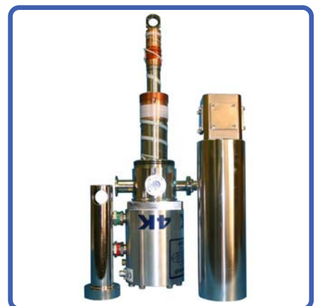
The above picture shows a coldhead, vacuum shroud, and radiation shield.
