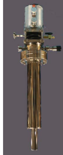
The vacuum shroud becomes narrow to permit sample insertion into a small magnet pole space.
