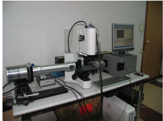
Micro PL. Adjustable sample to window distance for short focal length experiments.
