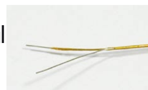
Kapton isolated Thermocouple
